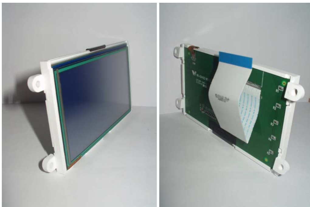
Figure 2. Custom designed LCD with integrated touch screen.
