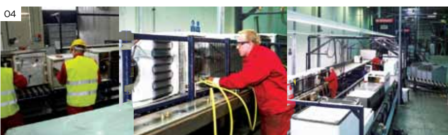
04 Opening an appliance on the recycling line: before the process certain components are removed manually; with refrigeration appliances the cooling circuit is removed as well as cooling gases and oil
