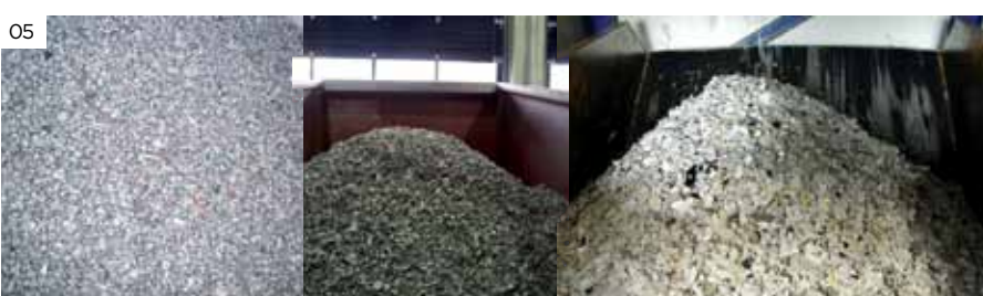
05 Separating metal, plastics, and other materials which are cut to required dimensions at the recycling centres
